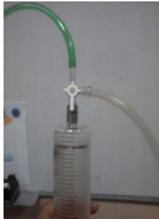
Gambar 7 Oil Flushing (pengambilan Oil Sample)
